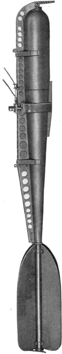
Trap, with bomb ready for release.
